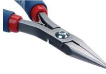
Features very fine tips, "eased" edges of the inner jaw to reduce the risk of damage to the workpiece during forming, and a long jaw for extended gripping power. Available with smooth or serrated jaws. Standard & Short Chain nose pliers have tips dimension of 1.2mm W x 1.4mm H (.050" x .060").
