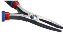
These flat nose pliers have a long jaw and very thin tips. The tip gripping area has a smooth finish. All inner edges are "eased" to reduce risk of workpiece damage. Standard flat nose pliers have tips that are 3.5mm (.140") wide and the Wide Tip Flat Nose Pliers have tips that are 6.3mm (.250") wide.
