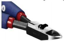
This cutter, forged of carbon steel, has strength in the head and joint areas needed to cut heavier gauge wire or cable. Cushion grips provide operator comfort. A jaw restraining device is attached to insure spring retention. Overall length 6" (152mm). Length of cutting blade 3/4" (19mm)
