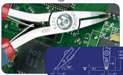
An SMT cutter with a very small cutting head. Used for exceptionally fine cutting. Relieved for maximum accessibility. Flush cutting edges.
