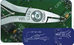
SMT Cutter. Extraordinarily small. Fine cutting edges and fine tip. Often used under a microscope. Removes individual leads from fine pitch components. Razor Flush<sup>™</sup> Cutting Edges.
